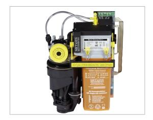
The MSTI is a single unit, two stage amalgam separator with an integrated air/water separation system and dental unit selector valve. The design of this super-reliable and safe amalgam separator has been proven by over 150,000 installations. The MSTI is ideal for daily use and can be installed inside your dental unit or in a separate cabinet. Product code 01010001: MSTI for installation in a dental unit. Product code 01010020: MSTI in floor-standing cabinet.
